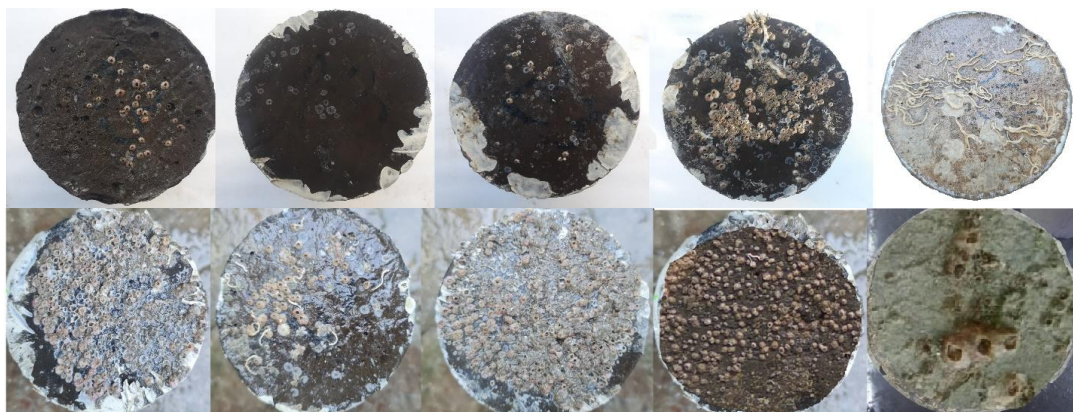
Fig. 8. Specimen surface after 30 days of immersion (top) and 150 days of immersion (bottom).
