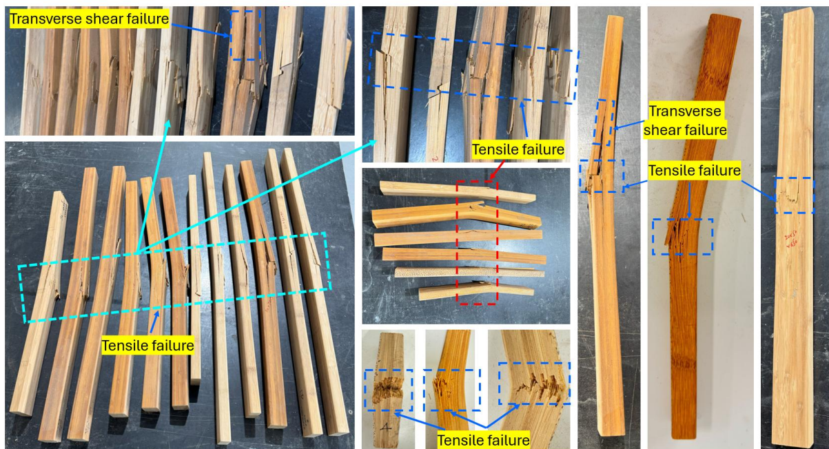
Fig. 3. Failure modes of long GLB compression elements with slenderness ratio ( \lambda \geq 38 )
