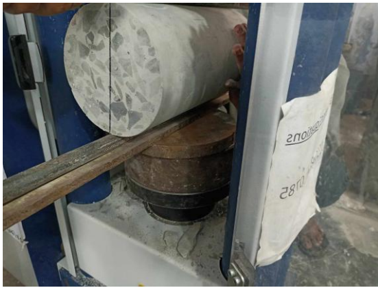
Fig. 3. Split tensile strength test
