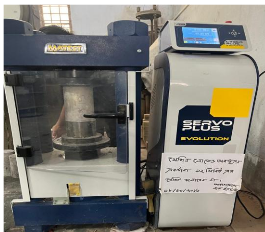
Fig. 2. Compressive strength test
