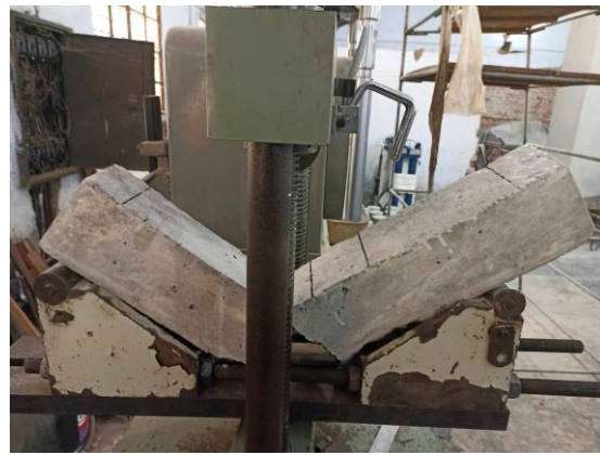
Fig. 4. Flexural strength test
