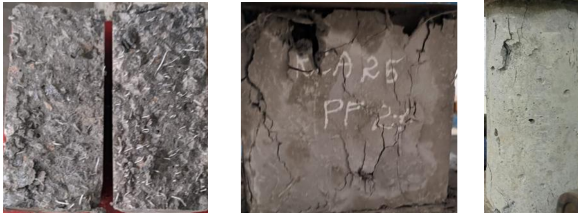
(a) Splitting tensile test (b) Cube Compression test (c) Uniaxial compression test
