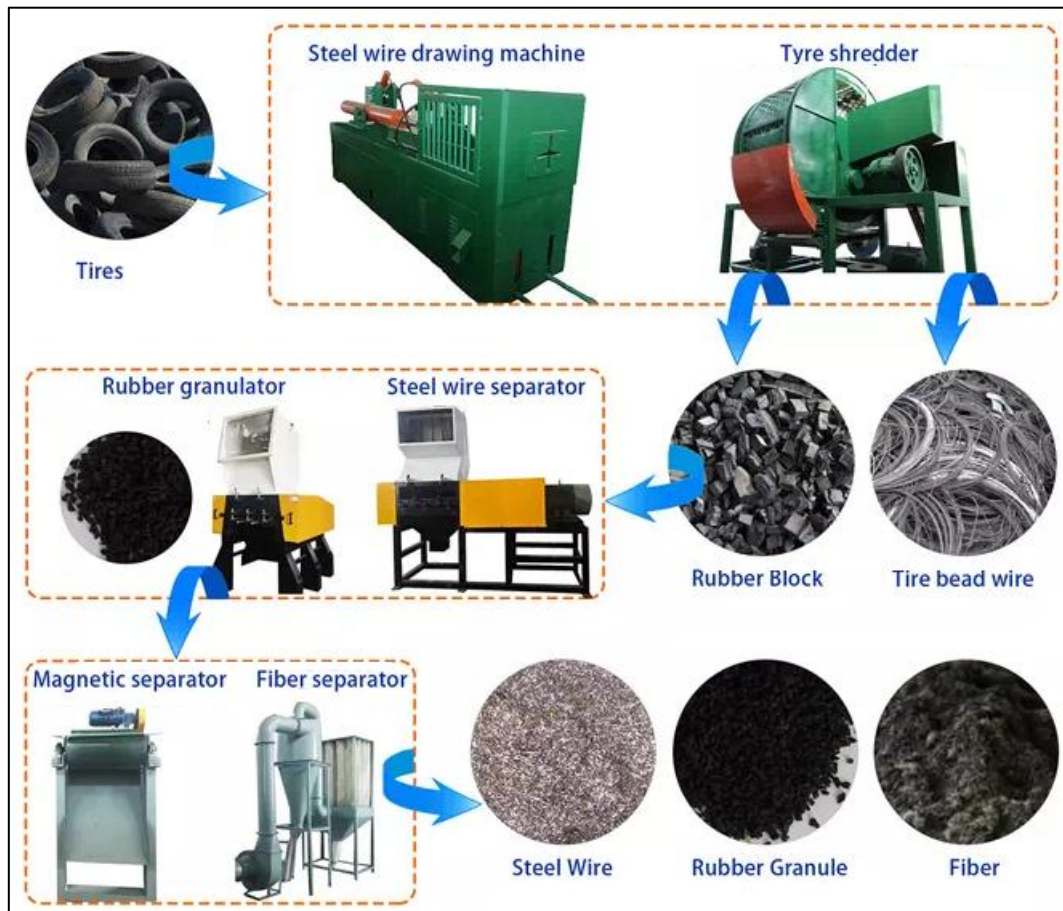
Fig. 4. Sketch of the scrap tire recycling processes (Adapted from an open access source [50])
