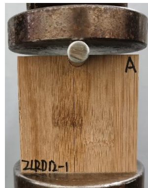
Fig. 3. The half-hole pin groove bearing test of laminated bamboo lumber
