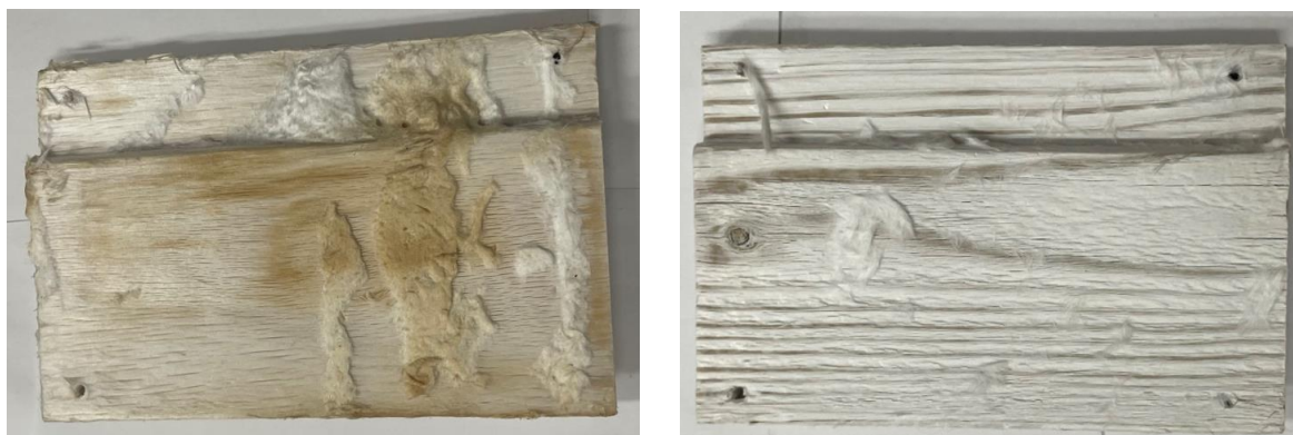
Fig. 11. Surface fibrillation observed after weathering in trembling aspen (left) and S-P-F (right) specimens.
