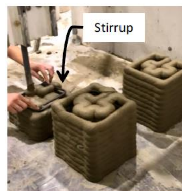
Fig. 1 (a) The Manufacturing process of post-tensioned 3D printed concrete girder [24]; (b) Steel reinforced 3D printed components [25].
