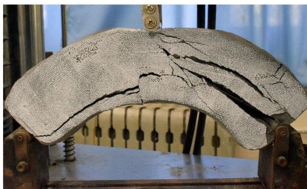
Fig. 5 Failure patterns of cable reinforced arch beam [40]
