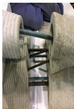
Fig. 1 (a) The Manufacturing process of post-tensioned 3D printed concrete girder [24]; (b) Steel reinforced 3D printed components [25].
