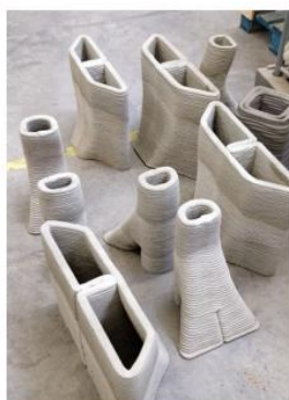
Fig. 1 (a) The Manufacturing process of post-tensioned 3D printed concrete girder [24]; (b) Steel reinforced 3D printed components [25].
