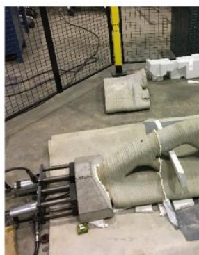
Fig. 1 (a) The Manufacturing process of post-tensioned 3D printed concrete girder [24]; (b) Steel reinforced 3D printed components [25].
